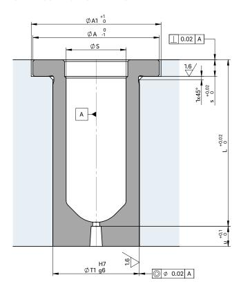
For gate bushings with an extended length, the gate contour goes through dimension "L"
